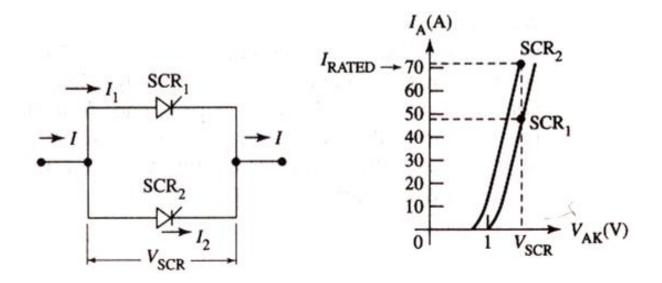
• Total rated current of parallel connection is  $I_1+I_2$ , not  $2I_2$ .
